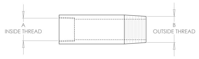
Use a tape measure to measure the outside or inside of the thread round up the measurement to the closest outside or inside diameter in the chart
