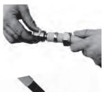
3) PUSH the fitting onto the tubing and fully <u>against the shoulder</u> of the fitting (soapy water will help this process)
