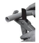
l) CUT the tubing square with the cutter, ROTATING wrist while cutting
