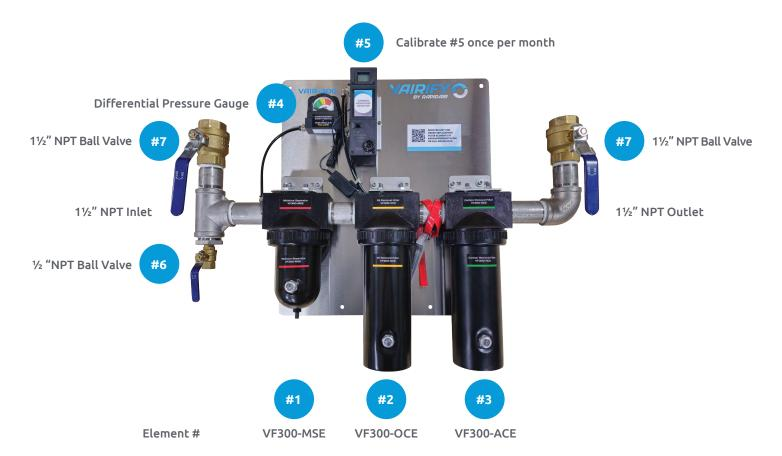
REPLACE ALL THREE FILTERS EVERY 6 MONTHS OR WHEN NEEDLE (#4) IS IN YELLOW DURING OPERATION (de-pressurize unit before changing filters)
