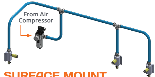
3/4" SURFACE MOUNT TUBING LAYOUT
